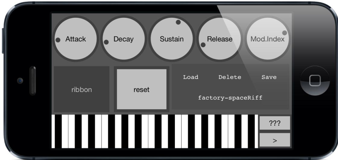
The four knobs in the upper left corner of the screen (“Attack,” “Decay,” “Sustain,” & “Release”) control parameters of **bent.fm lite**’s amplitude envelope generator (which is output by the ADSR chip).
